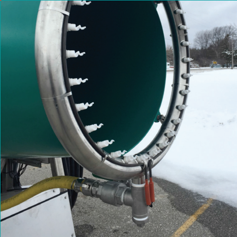
Heated spray manifold upgrade
